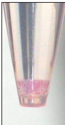
Figure 1: RalGDS RBD Agarose beads, in color, are easy to visualize, minimizing potential loss during washes and aspirations.
