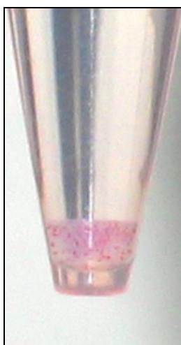
Figure 1: PAK RBD Agarose beads, in color, are easy to visualize, minimizing potential loss during washes and aspirations.
